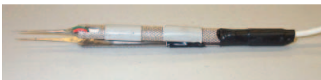
Figure 2 Forceps with strain gauges.
