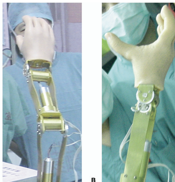
Figure 5. (a) The original position of the neural signal-controlled prosthesis. (b) Finger extension of the NSPSI was triggered during the operation.
