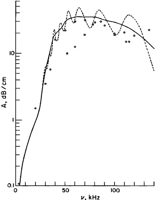
FIG. 13. Comparison between the attenuation coefficient given by (39) with the bubble distribution shown in Fig. 11 and the data of Ref. 14 (continuous line). The gas volume fraction is 0.02%. The dashed line has been obtained by using a bubble distribution consisting of a discrete number of sizes corresponding to the midpoints of the intervals of Fig. 11, rather than the continuous distribution of Fig. 11.
