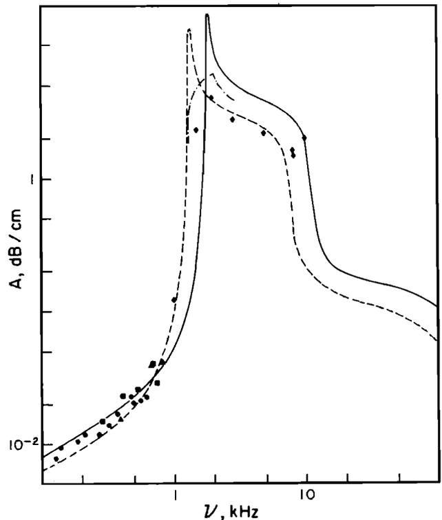
FIG. 3. Comparison between the attenuation coefficient given by Eq. (39) for a bubble radius of 1.77 mm (continuous line) and 2.44 mm (dashed line) and data from Ref. 13. The volume fraction is 0.22% and the bubble radii 1.77 mm (diamonds), 1.83 mm (circles), 2.07 mm (squares), and 2.44 mm (triangles). The dash-and-dot line is obtained with a constant distribution of bubble sizes between 1.77 and 2.44 mm normalized so as to give the correct volume fraction.
