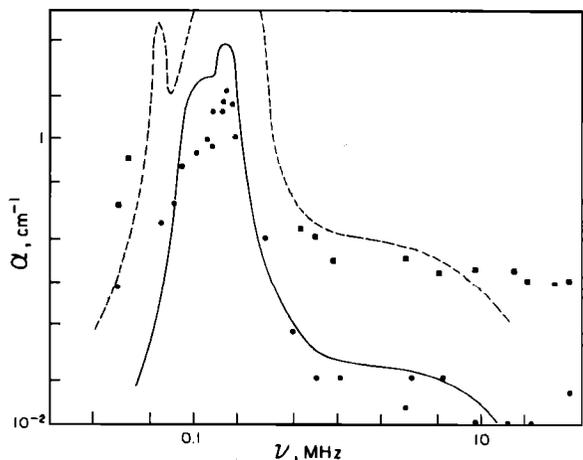
FIG. 17. Comparison between the attenuation length [given by Eq. (39) without the numerical factor 8.68589] for volume fractions of 0.004% (continuous line and circles) and 0.04% (dashed line and triangles) and data from Ref. 15. The continuous and dashed theoretical curves have been obtained using the continuous and dashed histograms Fig. 15, respectively.
