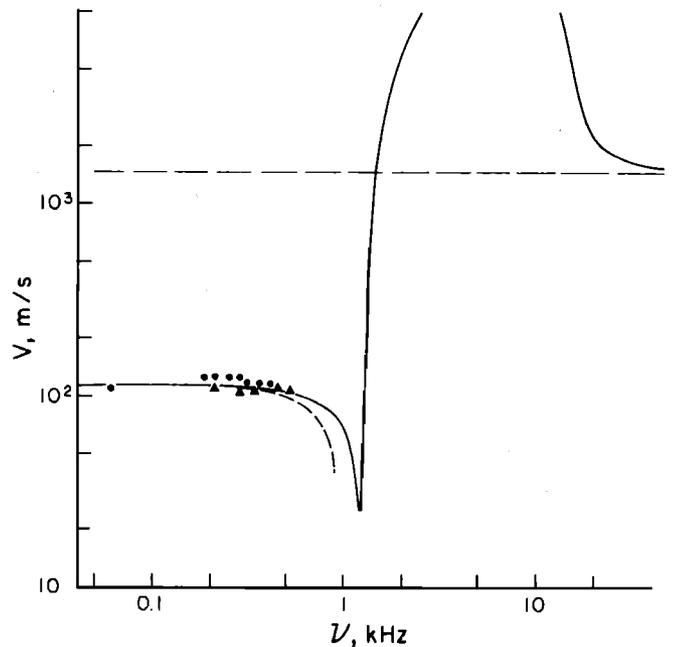
FIG. 10. Comparison between the phase speed of pressure waves given by (38) for a bubble radius of 2.68 mm and data from Ref. 13. The volume fraction is 1% and the data are for 2.68 mm (circles) and 3.64 mm (triangles). The dashed line is for a radius of 3.41 mm.
