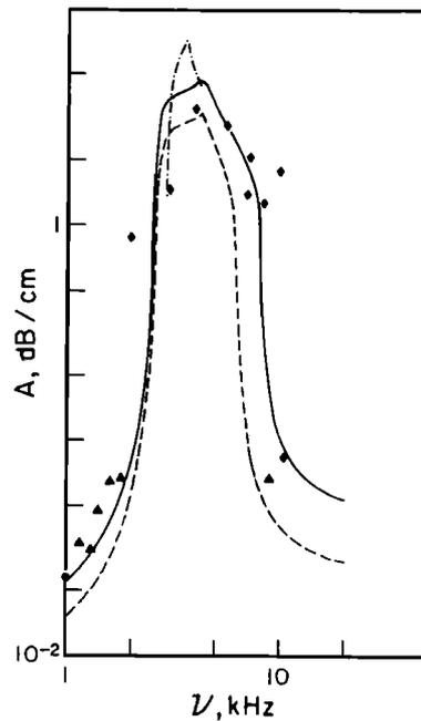
FIG. 2. The same data shown in the previous figure are compared here with the theoretical curves obtained by using the distribution function (63) with  $a_0 = 1$  mm,  $a_1 = 0.75$  mm,  $a_2 = 1.25$  mm,  $\sigma_a = 2$  mm, and with  $\beta = 0.0377\%$  (solid line) and  $\beta = 0.02\%$  (dashed line). The dash-and-dot line corresponds to the same distribution (63) but with a 10% spread in radii and, again,  $\sigma_a = 2$  mm,  $\beta = 0.0377\%$ .
