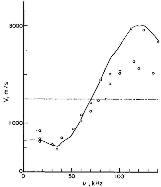
FIG. 12. Comparison between the phase speed given by (38) with the bubble distribution shown in Fig. 11 and the data of Ref. 14. The gas volume fraction is 0.02%. The dashed line is the phase speed in the pure liquid.
