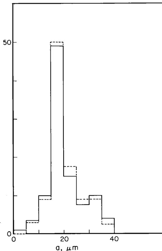
FIG. 14. Histograms of bubble sizes given in Ref. 15 for a liquid temperature of 15 °C and volume fractions of 0.02% (continuous line) and 0.03% (dashed line). The ordinate scale is in arbitrary units (different for the two lines).
