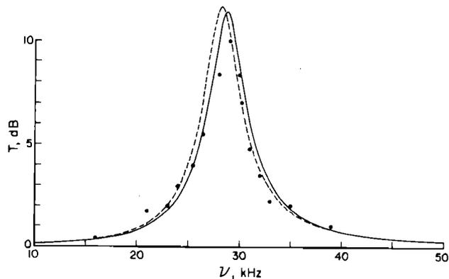
FIG. 19. Comparison between the transmission coefficient given by (55), in decibels, for bubbles with a radius of 0.110 mm (continuous line) and 0.112 mm (dashed line) and data from Ref. 16.
