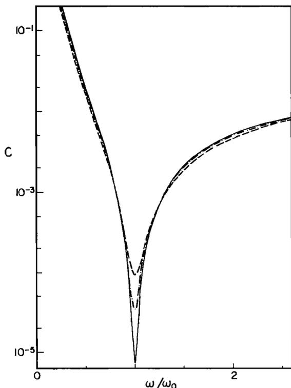
FIG. 22. Graph of the quantity defined in Eq. (66) as a function of the ratio of the driving frequency to the resonance frequency for bubbles with radii of 1 mm (continuous line), 0.1 mm (dash-and-dot line), and 0.01 mm (dashed line). These curves can be interpreted as an upper limit to the volume fraction for the validity of the present theory.
