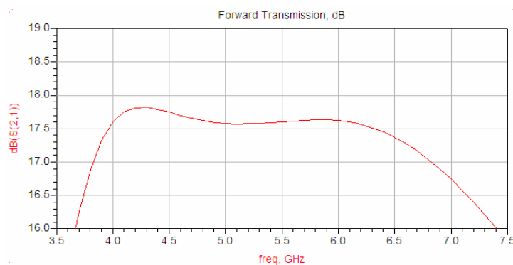
Figure 2: Simulation of S21 showing +/-0.5dB ripple from 3.7 to 6.8GHz.
