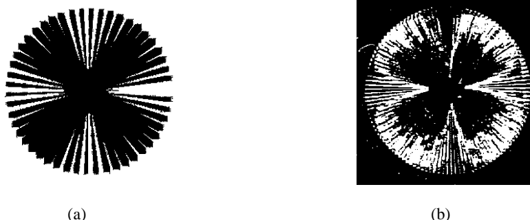
Fig. 4. Comparison of simulation and etching results using a spoke pattern. (a) simulation; (b) experiments.
