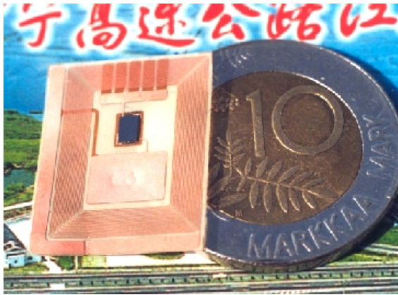
Fig. 2 Contactless RFID tag with ACF bonded Flip Chip
