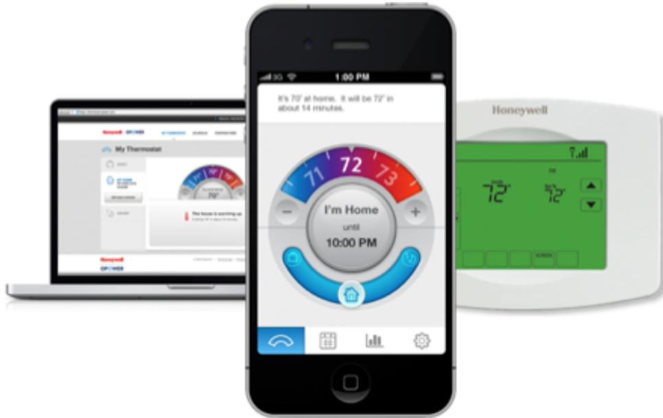
(a) Interfaces: The left panel shows the web portal, the middle panel shows the smartphone app, and the right panel shows the thermostat.
