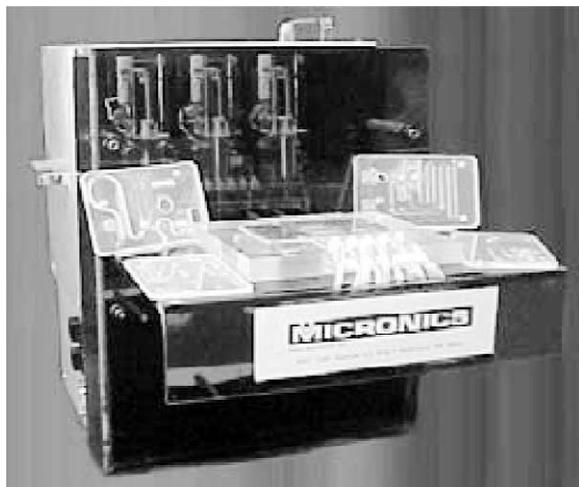
Fig. 6. Micronics liquid-liquid extraction platform, which uses laminar fluid diffusion interfaces to separate particles by size.
