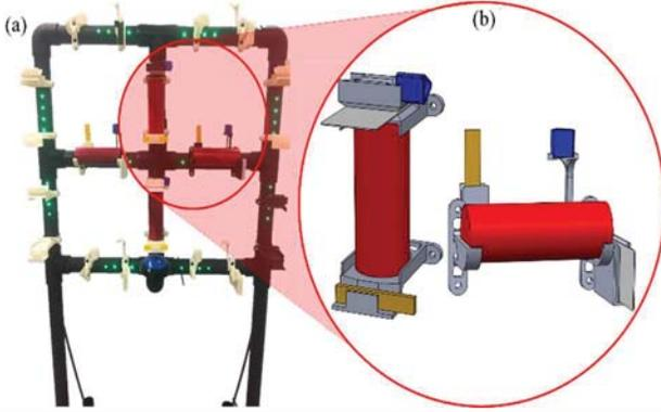
Figure 1: (a) An image of a complete PHAM windowpane. (b) Note that the horizontal and vertical testing environments are not the same. Slightly different designs are necessary to reduce the chance of collision while still guaranteeing each object can only be manipulated with one grip. The grip required to manipulate each primitive is represented by its color, the code of which can be found in Table I.
