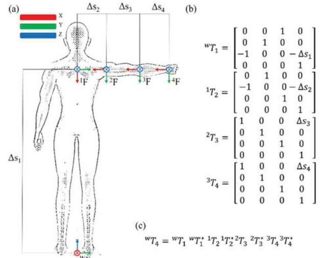
Figure 2: (a) The calibration pose with each IMU's ideal reference frame defined. (b) The ideal rigid body transformation relating each adjacent reference frame,  ${}^B T_A$ . (c) Hand position, in the world reference frame, is given by chaining these transformations with the calibration transforms,  ${}^B T_A^*$ .
