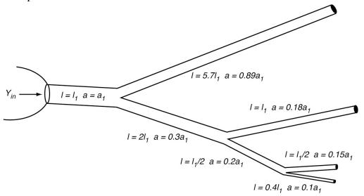
**Part a)** Write an expression for the input admittance  $Y_{in}$  of the tree, assuming that the tree is passive with open circuits ( $Y_L = 0$ ) at the ends of the terminal branches. There's an easy way and a hard way. Consider the equivalent cylinder.
