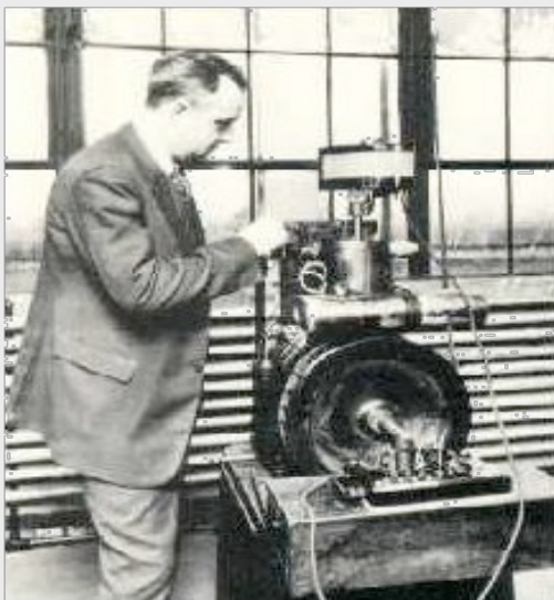
Thomas Midgley with the single cylinder laboratory engine used to test fuel additives.
